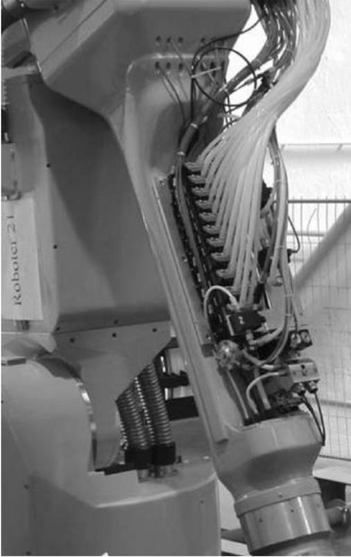
Fig. 8.13 Color changing installation in the robot arm.
