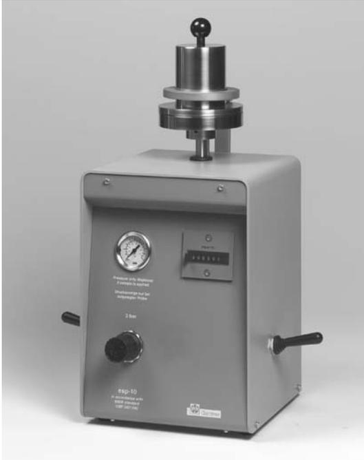
Fig. 12.75 Single-impact tester (source: Byk–Gardner).
