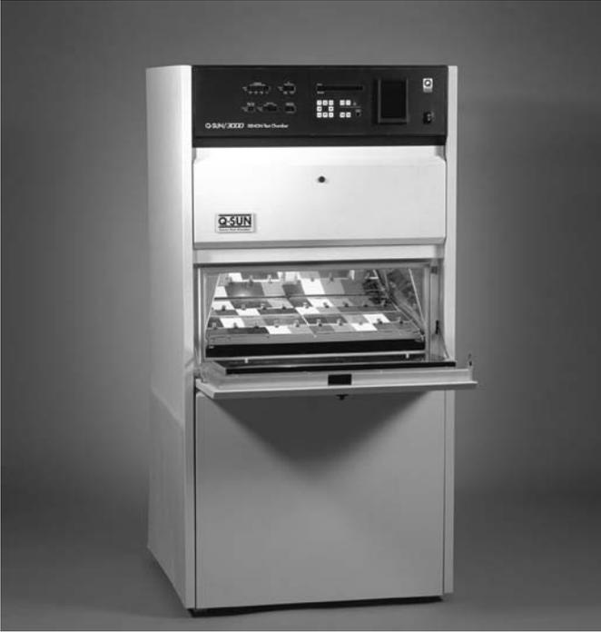
**Fig. 12.46** Example of a Xenon system with static sample arrangement.
