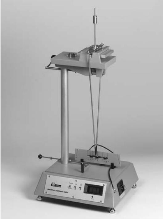
Fig. 12.59 König Pendulum damping device (source: Byk–Gardner).
