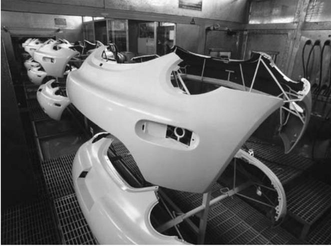
**Fig. 9.2** Painting of New Beetle bumpers (source: BASF Coatings).
