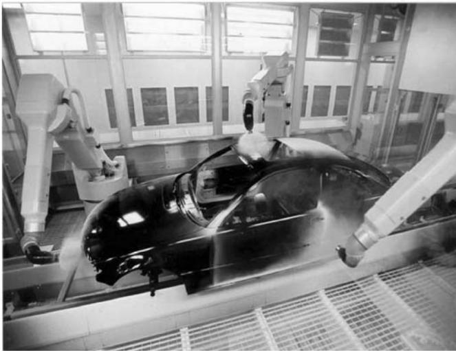
Fig. 8.4 Application of powder clear coats by robots and bells.
