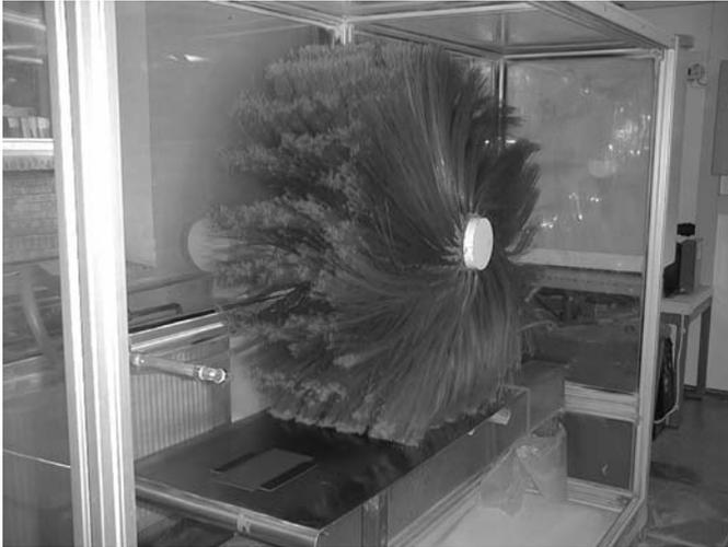
**Fig. 12.82** Car wash device from Amtec Kistler (source: DuPont Performance Coatings).
