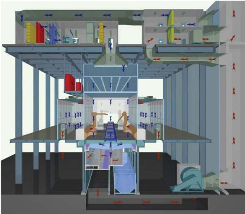
Fig. 8.8 Cross section of a spray booth.
