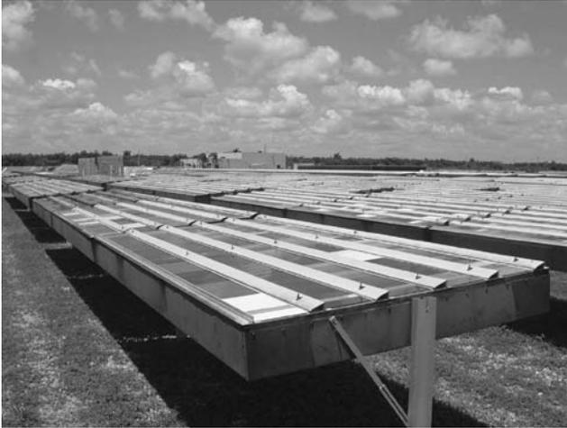
**Fig. 12.41** Black box for increased temperature of the panel during exposure.
