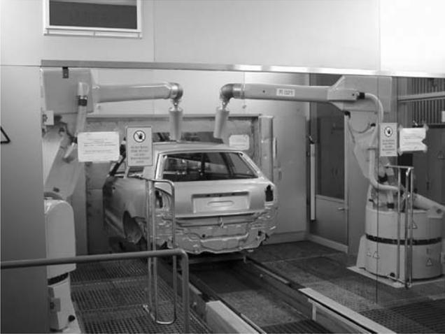
**Fig. 8.30** Robot-guided contactless online measurement of film thickness.
