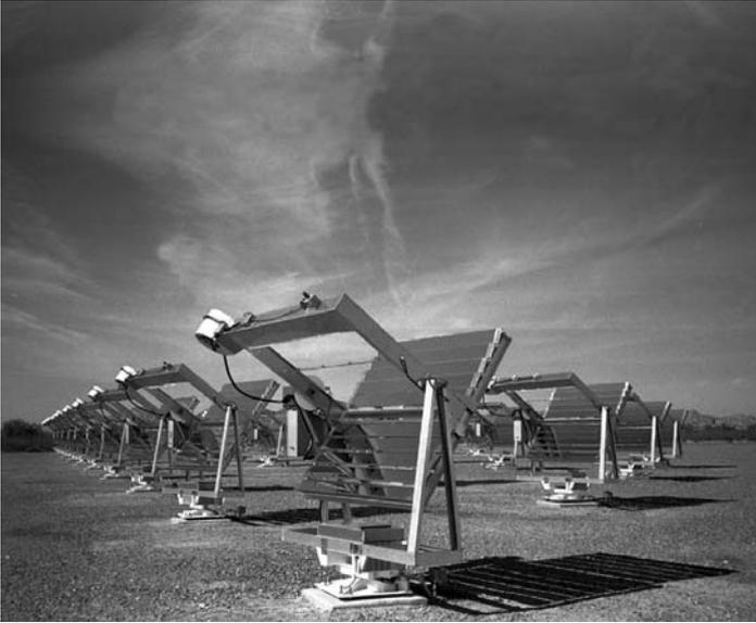
**Fig. 12.42** Example of a Q-track for increased irradiation of test panels.
