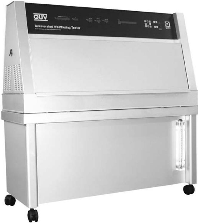
Fig. 12.48 Exterior view of a typical QUV tester.
