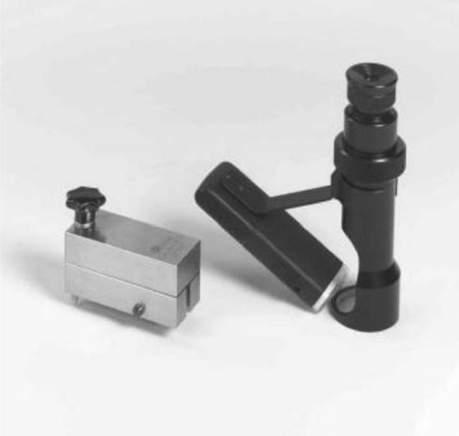
**Fig. 12.60** Buchholz test equipment (source: Byk–Gardner).
