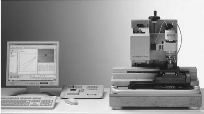
**Fig. 12.62** Total hardness measurement system
